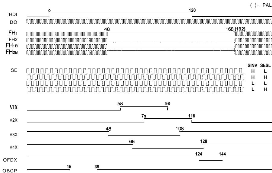
**"OFDX" PULSE TIMING < MIRROR, (MIR = H) >**
